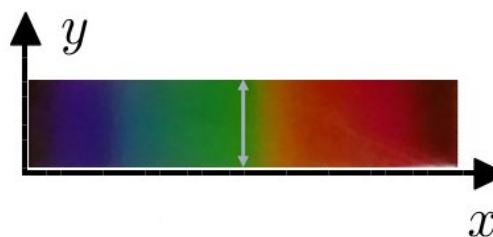
Figure 2. Exemplar LVF orientation with y-axis representing the linear uniformity and x-axis representing the linear thickness gradient.
