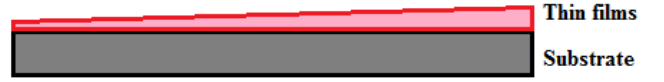
Figure 4. Thickness distribution of thin film layer on substrate produced using masks determined by simulation for accurate gradient structure.
