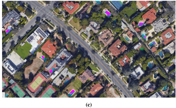
Fig. 9: a) Satellite imagery of the Beverly Hills Area (34.077566, -118.407321). b) Square SE used to detect swimming pools in the image. c) Detected swimming pools with P = 70\% overlaid onto the original.
